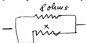
Suppose that a fixed 8-ohm resistor is connected in parallel with a variable resistor. If the resistance of the variable resistor is denoted by  $x$ , then the combined resistance  $R$  is a function of  $x$ . Graph  $R$  and give a physical interpretation of the graph.
